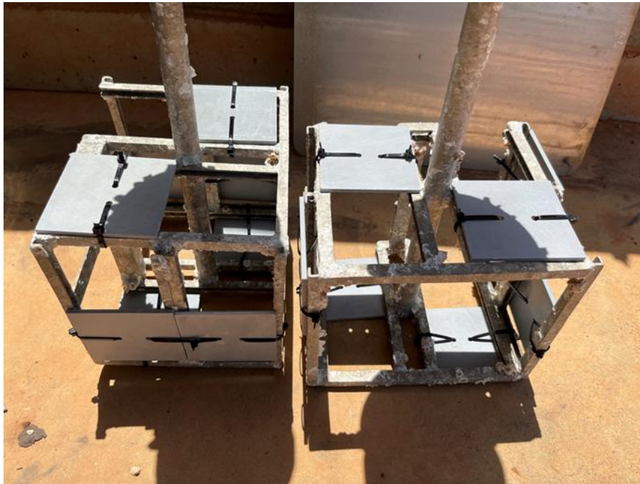
Arrays from State-Wide Array Surveillance program (SWASP) prior to two month soaking period under the wharf (Port of Broome)
