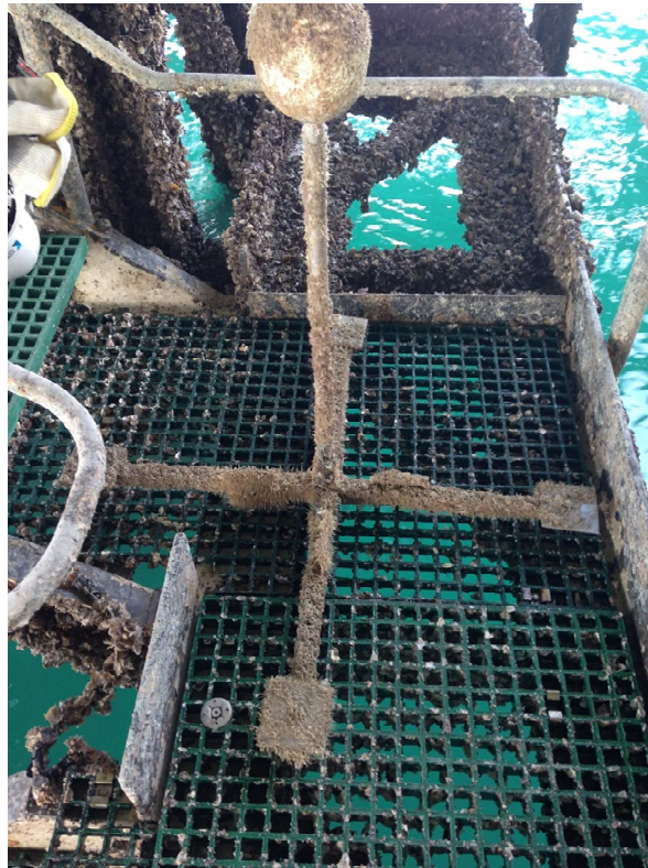
Array from State Wide Array Surveillance program (SWASP) after two month soaking period under wharf (Port of Broome)
